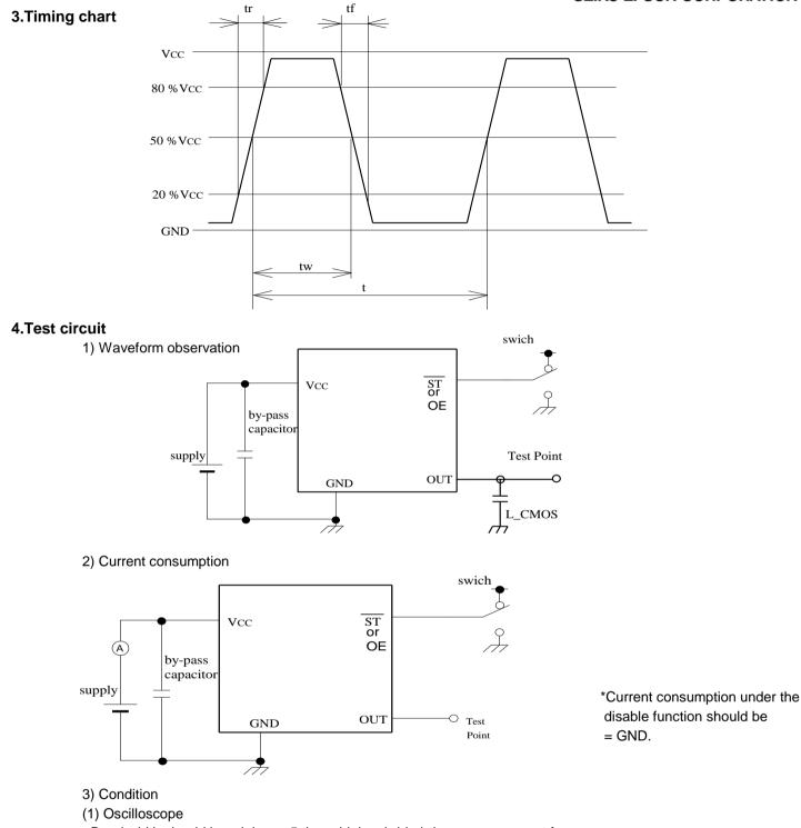
· Band width should be minimum 5 times higher (wider) than measurement frequency.
